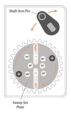
a. Using a Phillips head screwdriver, remove the two screws holding the sweep set plate to the gear wheel and then rotate the Sweep Set Plate a full 180°, reloacating the desired sweep set hole over the oblong slot on the opposite side of the wheel.
