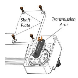
a. Using the provided Allen wrench, remove the four screws from the shaft plate and carefully remove the shaft plate.
